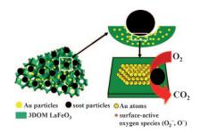
The catalyst support 3DOM LaFeO $_3$  contains highly ordered macropores that are connected with each other by small windows. 3DOM LaFeO $_3$  supported gold catalysts, which combine the advantages of good contact by the macroporous support and highly active sites for activation of O $_2$  by gold clusters, exhibit super catalytic performance for soot oxidation.
